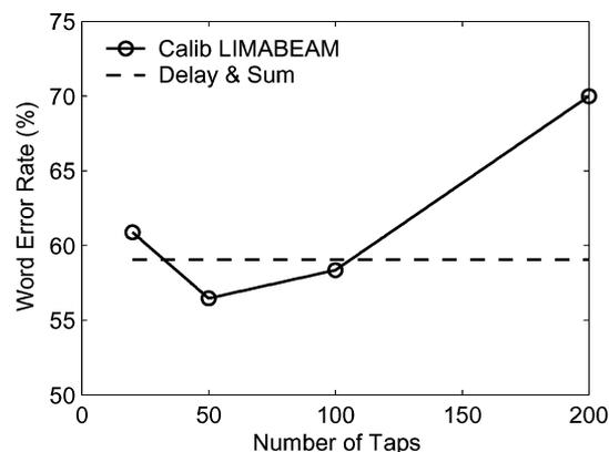
Fig. 1. WER as a function of filter length for the WSJ<sub>0.47</sub> corpus when the filter parameters are optimized using Calibrated LIMABEAM. The performance using conventional delay-and-sum processing is also shown.
