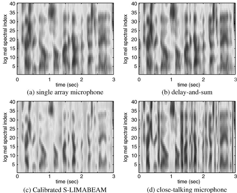
Fig. 4. Log mel spectrograms of a segment of an utterance from the WSJ<sub>0.47</sub> corpus obtained from (a) a single channel in the array, (b) delay-and-sum beamforming, (c) the Calibrated S-LIMABEAM algorithm with five taps per filter, and (d) the close-talking microphone signal.
