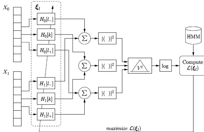
Fig. 2. S-LIMABEAM for an array of two microphones for the  $l$ th log mel spectral component which is composed of three subbands.  $X_0$  and  $X_1$  are the STFT vectors for microphones 0 and 1, respectively, and  $V^l$  is the  $l$ th mel filter.
