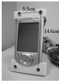
Fig. 3. Four-microphone PDA mockup used to record the CMU WSJ PDA corpus.
