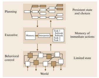
Fig. 8.4 Prototype three-tiered architecture
