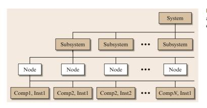
Fig. 8.7 The JAUS reference architecture topology (after JAUS Reference Architecture document [8.63])
