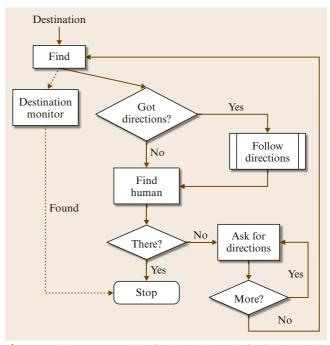
Fig. 8.11 Finite-state machine for GRACE's task for following directions to the registration booth
