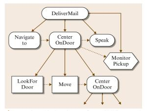
Fig. 8.8 Hierarchical task tree for mail-delivery task (lozenge nodes are interior; rectangular nodes are leaves; hexagonal node is an execution monitor; solid arrows are parent-child relationships; dashed arrows are sequential constraints)
