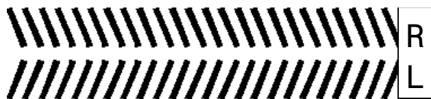
Figure 10: (R, L) states of louver filter. In R state, bias favors the right eye, in the L state it favors the left eye.
