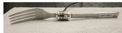
Figure 4.7: Force-torque sensor embedded within a fork to measure forces and torques applied at the tinetips.
