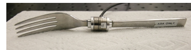
Figure 4.3: Fork with infrared markers mounted on the opposite end from the fork tines.
