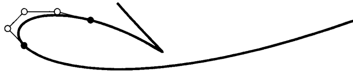
Figure 5.3 Convex hull property: a quartic Bézier curve is plotted for parameter values t \in [-1, 2] .
