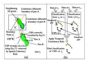
Figure 5. (a) Spatial coherency removes spurious segmentation errors, (b) Temporal consistency ensures segmentation agrees between successive frames.
