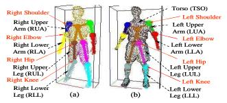
Figure 7. Complete articulated human model of (a) the synthetic data set (different body parts shown with different colors), (b) the real person. These are the models used for motion tracking in the experimental results in Section 4.3.
