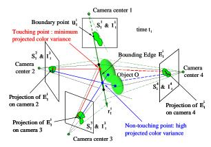
Figure 1. The Bounding Edge  $E_1^i$  is obtained by first projecting the ray  $r_1^i$  onto  $S_1^2$ ,  $S_1^3$ ,  $S_1^4$  and then re-projecting the segments overlapping the silhouettes back into 3D space.  $E_1^i$  is the intersection of the reprojected segments. The point where the object touches  $E_1^i$  is located by searching along  $E_1^i$  for the point with the minimum projected color variance. Note that the image from camera 4 is not used because it is occluded. See [4] for details.
