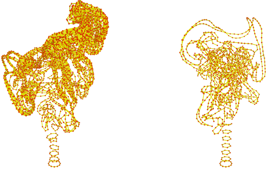
Figure 2: Without reconnection, thick bundles of vortex filaments form ( left ). With reconnection, the simulation contains \frac{1}{3} the number of filaments, though a small amount of viscosity is introduced ( right ).
