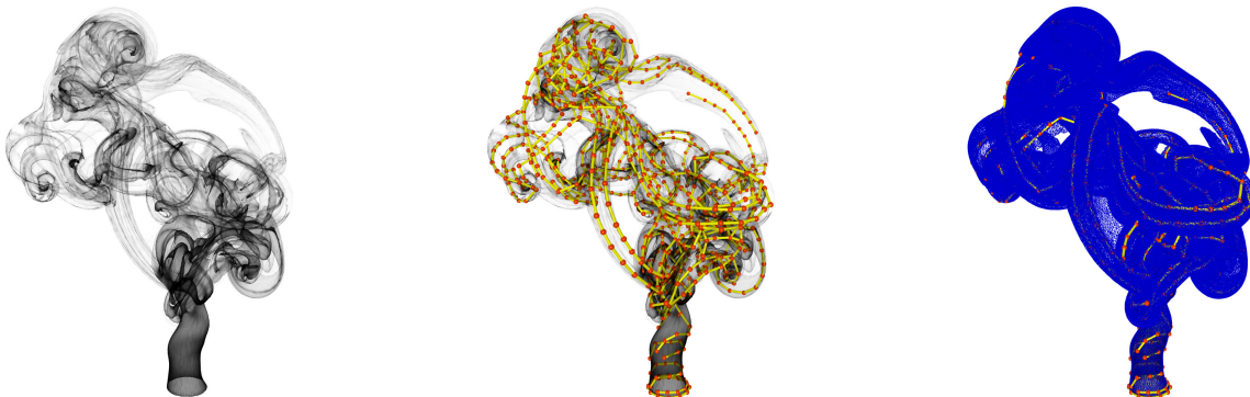
Figure 1: A smoke plume simulated using our method ( left ). Fluid motion is simulated using vortex filaments ( center ) and the smoke surface is tracked using a triangle mesh ( right ).
