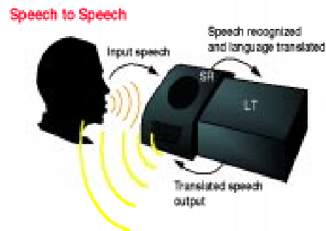
Fig. 7. Speech Recognizer (SR) and Language Translator (LT) Smart Module
