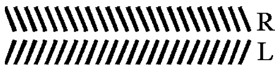
Fig. 10. ( R , L ) states of louver filter. In R state, bias favors the right eye, in the L state it favors the left eye.
