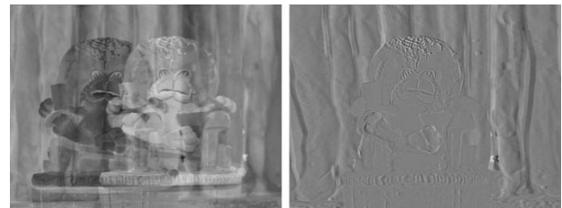
Fig. 6. Gray-level representations of disparities (differences) between the image pairs of Figs. 4 and 5. When corresponding pixels are identical, this representation is midrange gray; negative (left–right) differences are darker, positive differences lighter.
