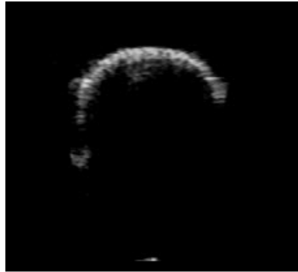
Figure 5. An ultrasonic image after correction for focussing effects of the transducer and lensing effects of the plastic tube. The correction is linear with depth. The widths are also scaled so that objects at TV line 167 (4cm) are the same width in the corrected image as they are in the original image.
