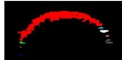
Figure 7. Regions in an ultrasonic image. Each region has a different color. Only the largest regions are used to establish a contour. Smaller ones are deleted ("culled").
