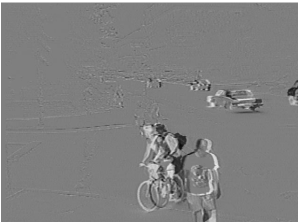
Fig.7a: Frame difference between a T2 and a B frame
