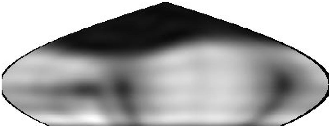
**Figure 9:** dual filament bulb, high beam, regenerated and interpolated data, 1x1 grad steps
