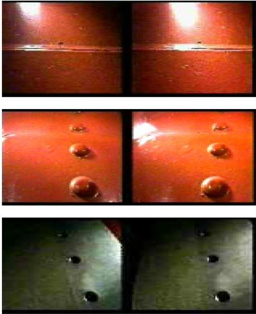
Fig. 9: Three left and right eye 3D-stereoscopic views from the 4.5x 3D-stereoscopic camera in the sensor pod. Top is a lap joint, middle is a row of buttonhead rivets, bottom is a sheet metal sample from a “defect library.” Note, in addition to the perspective differences between the two views (which stimulates depth perception), the distinct differences in specular reflections (which we believe stimulates texture recognition).
