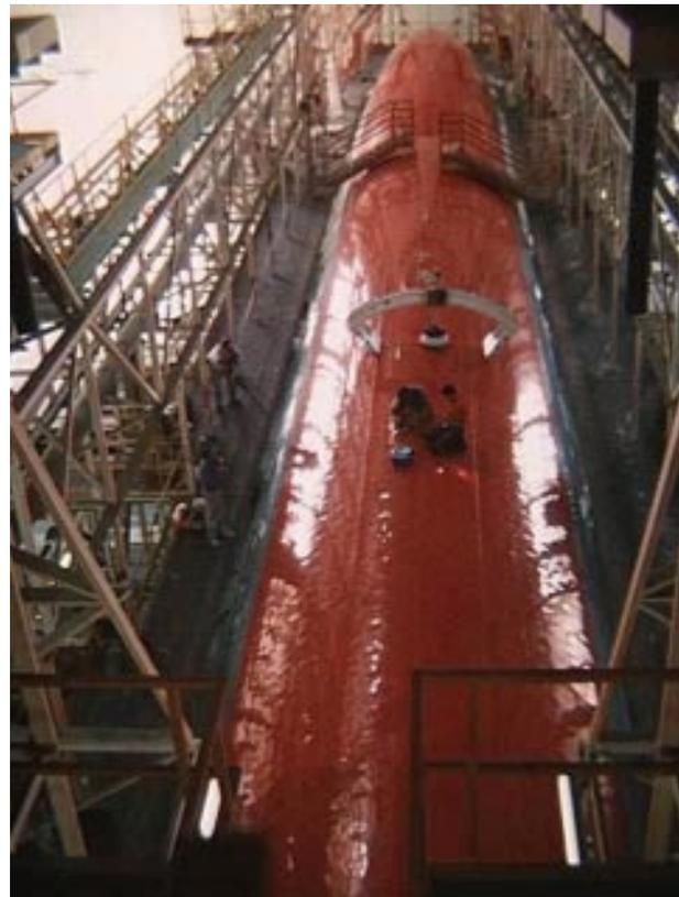
Fig. 5: CIMP on a 747 in a heavy maintenance bay at Northwest Airlines Minneapolis headquarters. The inspector, observed by a CMU staffer, is performing an eddy current check of a visual anomaly detected using the remote vision system shown in Fig. 7. Future models would incorporate remotely operated eddy current sensing.
