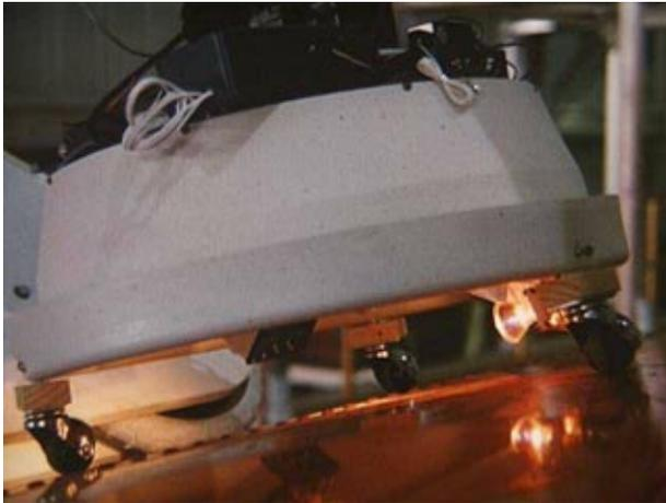
Fig. 7: Sensor pod, showing 3D-stereoscopic camera (white box with black endcap left of and below center) and remotely movable low angle illuminator. Inspector can remotely swing this illuminator in a 300 degree arc centered on the forward viewing direction of the camera, reproducing the way he typically uses his flashlight to pick up highlights. The flood illuminator is not visible in this view.
