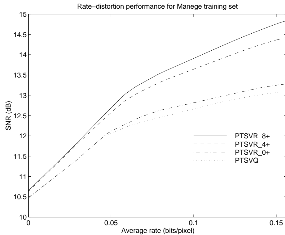
Figure 5.5: PSNR vs. average rate for Manege training set, a) balanced, binary trees, b) length-pruned trees.
