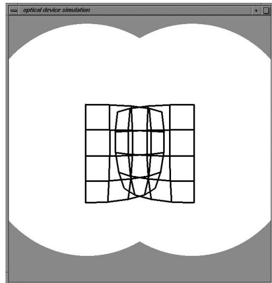
**Figure 10:** 2 lenses, barrel distortion ( $E > 0$ )
