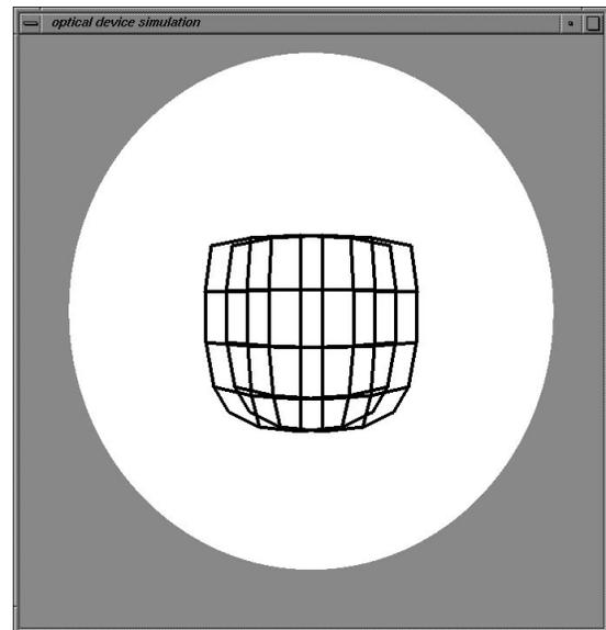
**Figure 6:** 1 lens, barrel distortion ( $E > 0$ )
