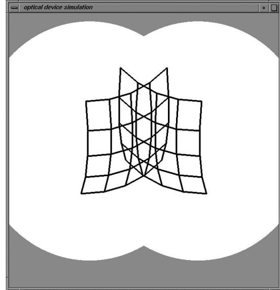
**Figure 8:** 2 lenses, pure curvature-of-field ( $D \neq 0$ )
