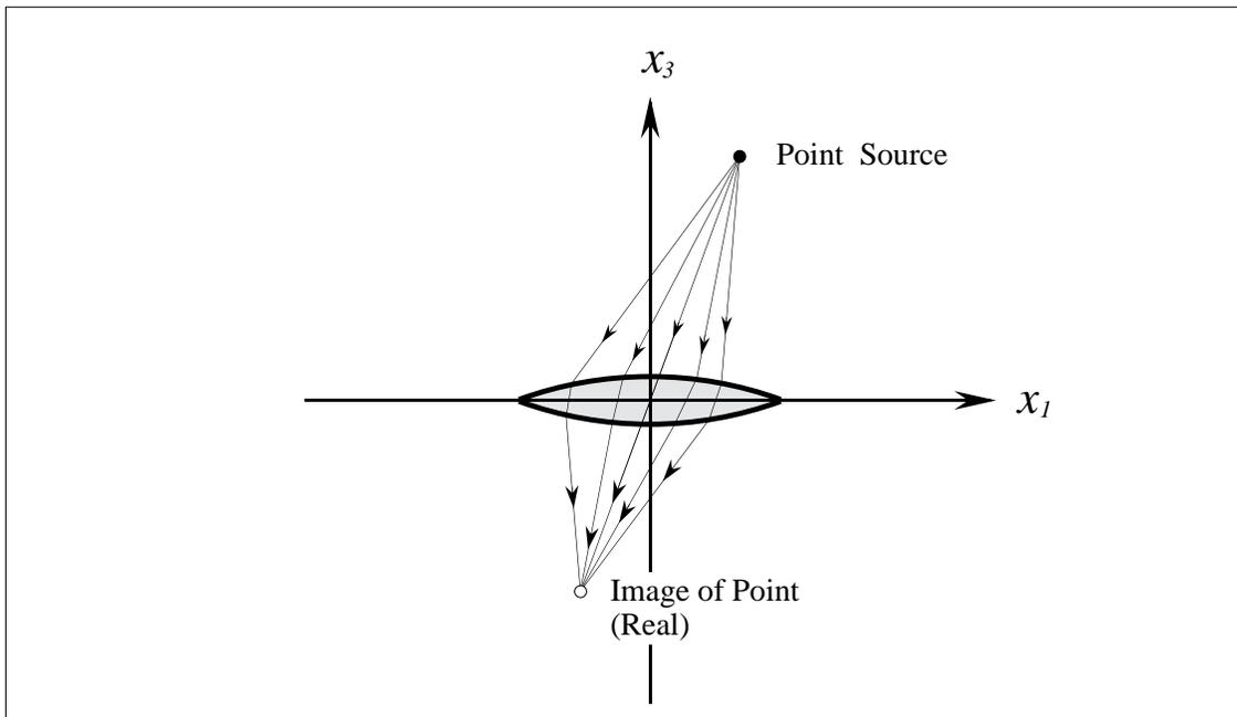
**Figure 4. A lens as an ideal optical device.**
