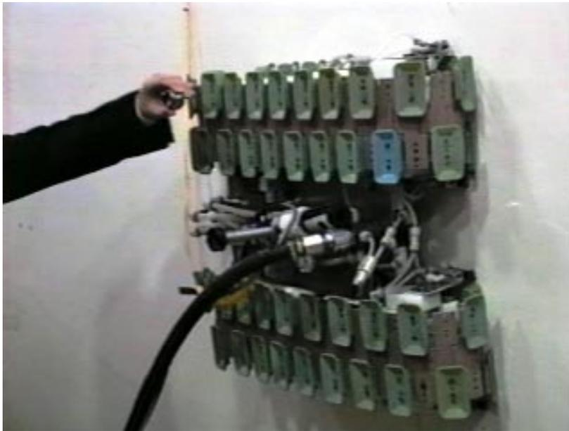
Fig. 3: AutoCrawler on the side of an airplane. The hand is about to install, on the "periscope" at the center of the AutoCrawler, a retroreflector that is part of the laser tracking system used for locating the robot absolutely relative to the hangar floor.
