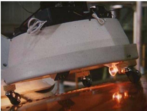
Fig. 6: Sensor pod, showing 3D-stereoscopic camera (white box with black endcap left of and below center) and remotely movable low angle illuminator.
