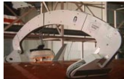
Fig 2. Crown Inspection Mobile Platform (CIMP) robot
