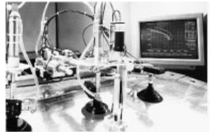
Fig 1. Automated NonDestructive Inspection (ANDI) robot
