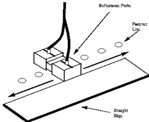
**Figure 2:** "Reflectance" or "pitch-catch" eddy current probe.
