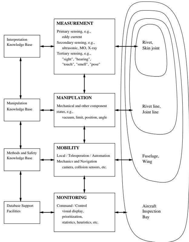
Figure 1: The 4M-s of automation for aircraft inspection.
