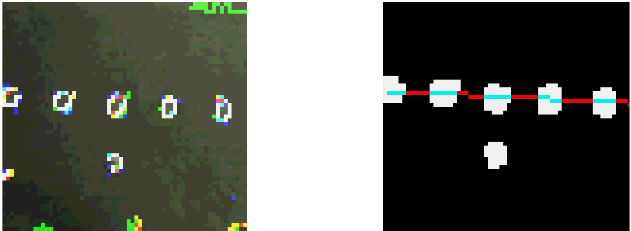
FIGURE 2. (a) Results of running Canny edge detector on all three color bands separately. The five bright regions in a row in the middle of the image and the one bright region in the middle below the third region in the row are rivets. (b) Result of heuristic blob evaluation and robust line fitter; the outlying rivet does not affect the line.
