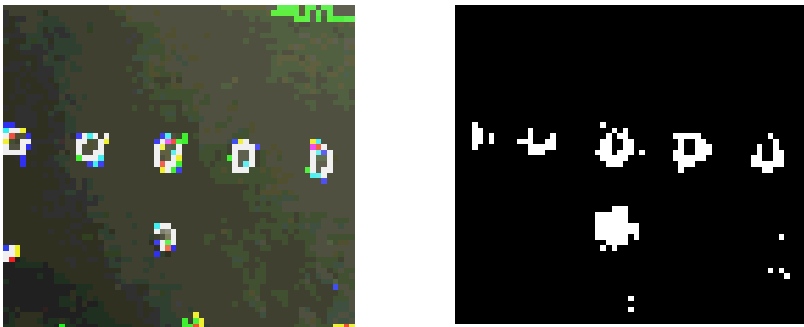
FIGURE 6. (a) Edges found with Canny operator. (b) Edges found with neural edge detector.
