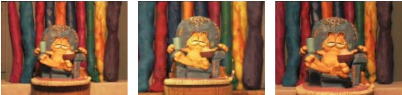
**Figure 1. Pictures of the same scene with telephoto (left), normal (middle), and wide-angle (right) lenses at corresponding long, intermediate, and short distances from camera to scene. Notice “flatness” at left, “depth” at right.**
