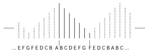
Fig. 6. Periodic symmetric extension of a signal
