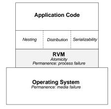
Figure 2: Layering of Functionality in RVM
