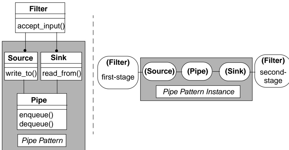
**Figure 5: OMT-based specification of simple pipe-and-filter system architecture. The pipe connector is represented as a design pattern. Connector interfaces (source and sink) are now first-class entities.**
