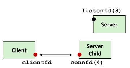
3. Server returns connfd from accept. Forks child to handle client. Connection is now established between clientfd and connfd
