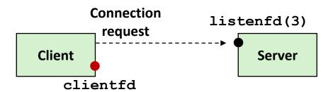
2. Client makes connection request by calling connect
