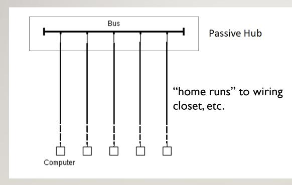
The bus remains an equivalent collision/contention domain, but the wiring gets easier, physically.
