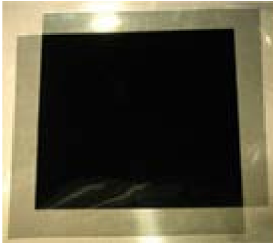
Light Passing Through Crossed Polarizers
