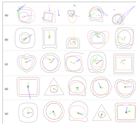
FIGURE 28. Learning the And-Or graph parameters for the clock category. (a) Sampled clock examples (synthesis) based on SCFG (Markov tree) that accounts for the frequency of occurrence. (b-e) Synthesis examples at four incremental stages of the minimax entropy pursuit process. (b) Matching the relation positions between parts, (c) further matching the relative scales, (d) further pursuing the hinge relation, (e) further matching the containing relation. From [49]
