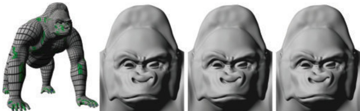
Fig. 11. A complex mesh with boundary. From left to right: Catmull-Clark patch structure, Geometry patch approximation, Geometry/Tangent patch approximation and Catmull-Clark limit surface.
