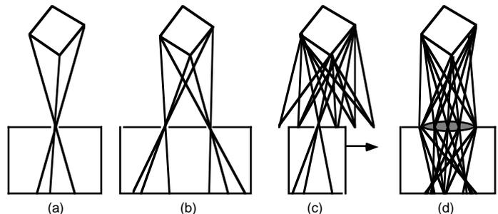
Fig. 2. (a) Pinhole camera forms an image from a single viewpoint; (b) in a stereo system, two images are formed from different viewpoints; (c) in a motion parallax system, a sequence of images are captured from many adjacent viewpoints; (d) a lens gathers light from a continuum of viewpoints; in an ordinary camera these images are averaged at the sensor plane.
