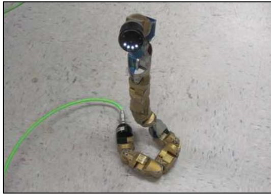
Figure 1. Snake robot performing inspection: tail and base links provide support while the head (containing the camera) and the body of the snake rise into the air to scan the environment.
