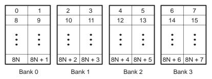
For devices that have more than one memory space (Figure 4–2), an access to bank 0 in one memory space does not interfere with an access to bank 0 in another memory space, and no pipeline stall occurs.
