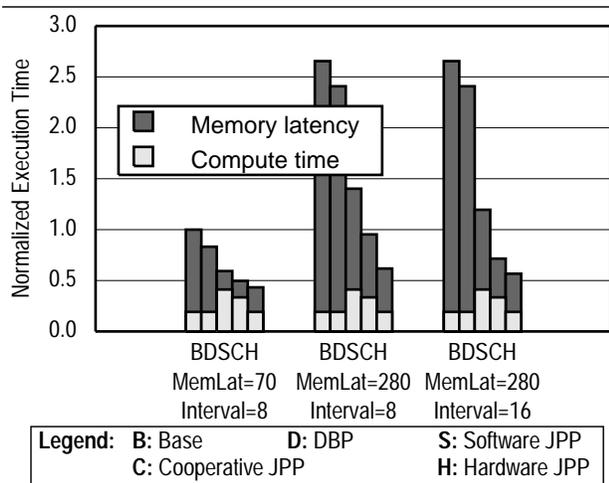
**Figure 7. Tolerating longer memory latencies.** Execution times for health: the first group of bars uses the base configuration (70 cycle memory latency), the second and third simulate long memory latency (280 cycles). In terms of prefetching, the first two configurations use a jump interval (the distance between a jump-pointer’s home and target nodes) of 8, the third uses an interval of 16.
