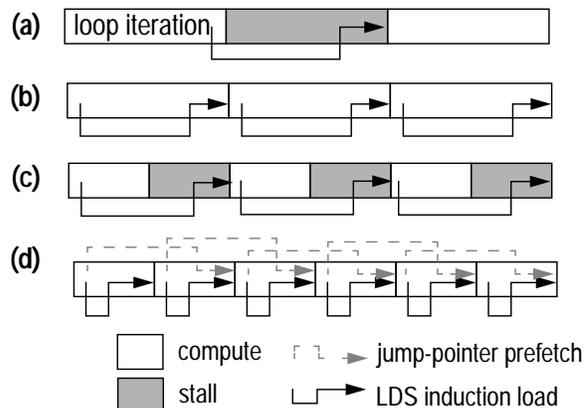
**Figure 1. Hiding LDS load latency.** (a) Exposed induction load latency can be hidden by (b) scheduling it early in an iteration. (c) This approach is ineffective if a single iteration has insufficient work. (d) Jump-pointers can leverage the work of multiple iterations.
