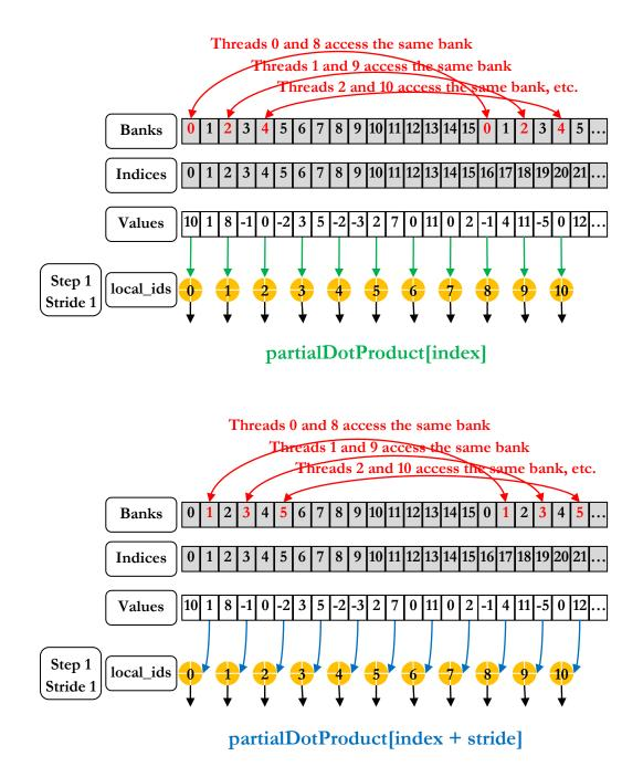
Figure 5. partialDotProduct[index] and partialDotProduct[index + stride] from kernel of Listing 5 exhibit 2-way bank conflicts (showed for Step 1 in this figure).
