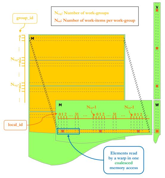
Figure 3. A work-group computes multiple elements of W (one every  $N_{wg}$  elements). Global memory accesses are coalesced.
