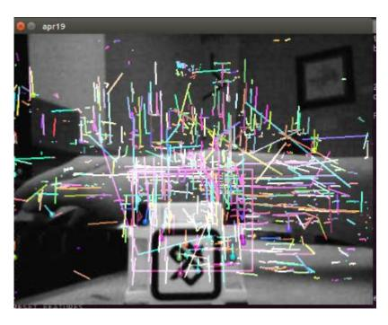
Optical flow returns distance between similar points in adjacent frames. Obstacle detection occurs in a small region in front of the robot
