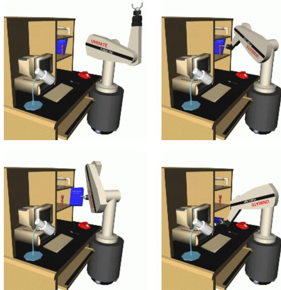
Figure 9: Path planning for a 6-DOF Puma robot.
