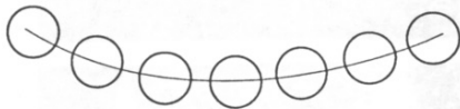
FIGURE 4b. Strobing occurs in a faster action when the object's positions do not overlap and the eye perceives separate images.
