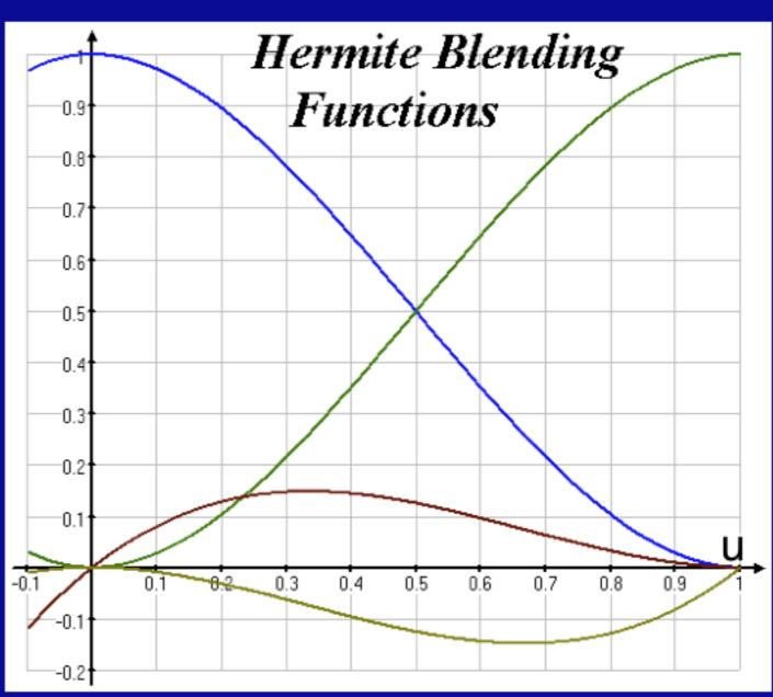
Every cubic Hermite spline is a linear combination (blend) of these 4 functions
