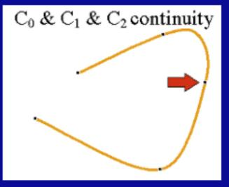
Continuous in position, tangent, and curvature
