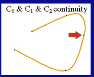
Continuous in position, tangent, and curvature
