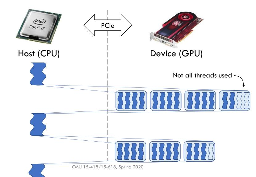
Setup memory (from CPU to GPU)
