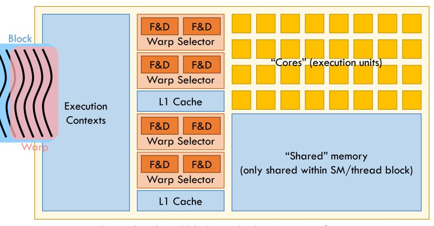
Within an SM, thread blocks are broken into warps for execution
