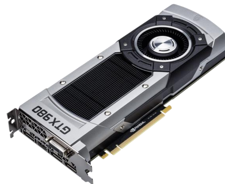
GTX 980: 16 SMM cores (165 watts)
