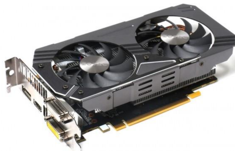
GTX 950: 6 SMM cores (90 watts)
