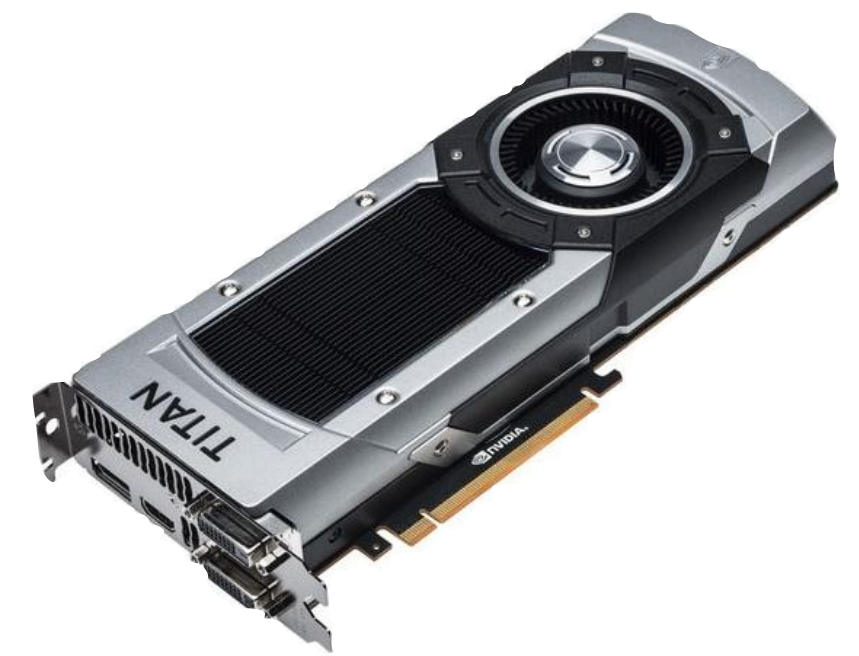
Titan X: 24 SMM cores (250 watts)
