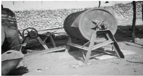
Figure 3: A ball mill being used as part of a gold mining operation in Arequipa, Peru
