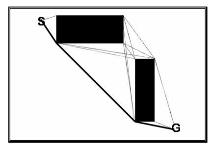
1. (5 points) The initial visibility graph is shown with dotted lines. The path found from start (S) to goal is shown with solid lines.
