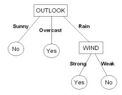
The test set accuracy is  $\frac{5}{7}$ . In this case, the tree built was too general. In particular, the training set did not include examples where the sunny attribute was positive. Therefore, the model failed to classify such instances in the test set.
