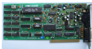
1989 Sound Blaster 1.0 11 voice FM synthesizer
