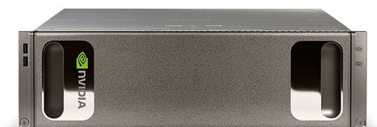
Nvidia DGX-1 8x Tesla V100, 3.2 kW 170 Tflop/s FP64, 1Pflop/s FP16, 128 GB
