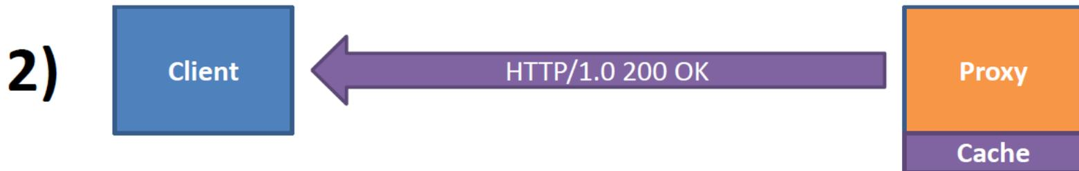
The Proxy simply responds with the stored result for `http://www.google.com/`. The Client is unaware that it has not communicated with the `google.com` server directly.
