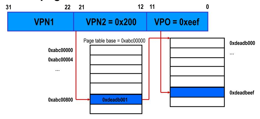
Use the second VPN to index into the page table. This gives the address of the start of the page frame. Add the offset to obtain the location in physical memory.
