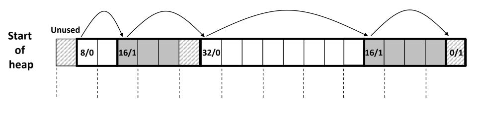
Double-word aligned Allocated blocks: shaded Free blocks: unshaded Headers: labeled with size in bytes/allocated bit
