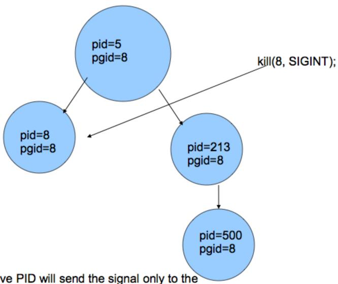
kill() with a positive PID will send the signal only to the process with that ID.
