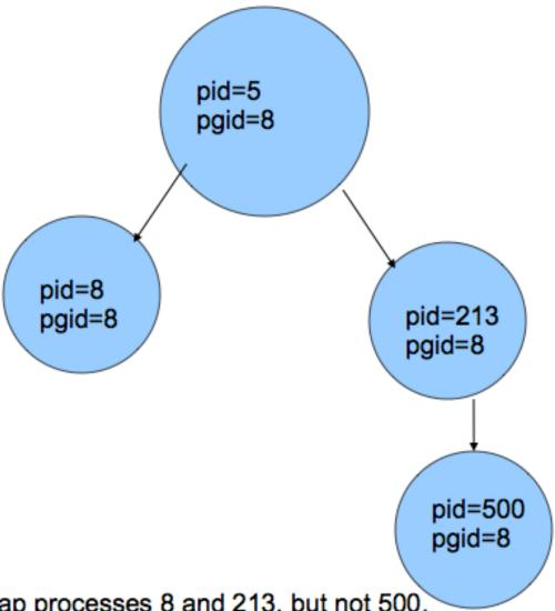
process 5 can reap processes 8 and 213, but not 500. Only process 213 can reap process 500.
